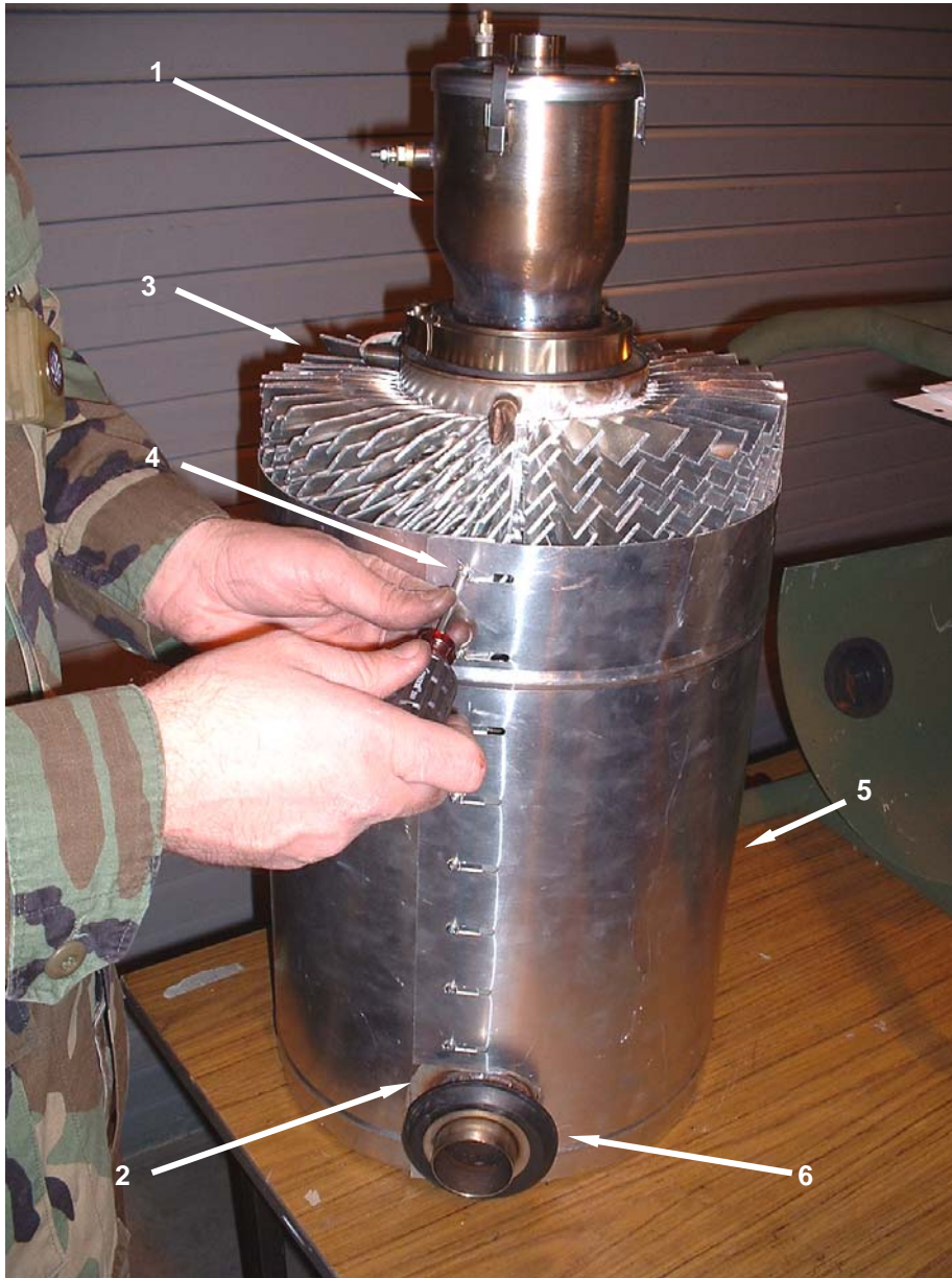
Figure 6. Replace Fin Temperature Sensor – Remove Wrap Cover.
