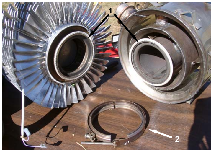
Figure 3. Inspect Thermoelectric Generator (TEG).
