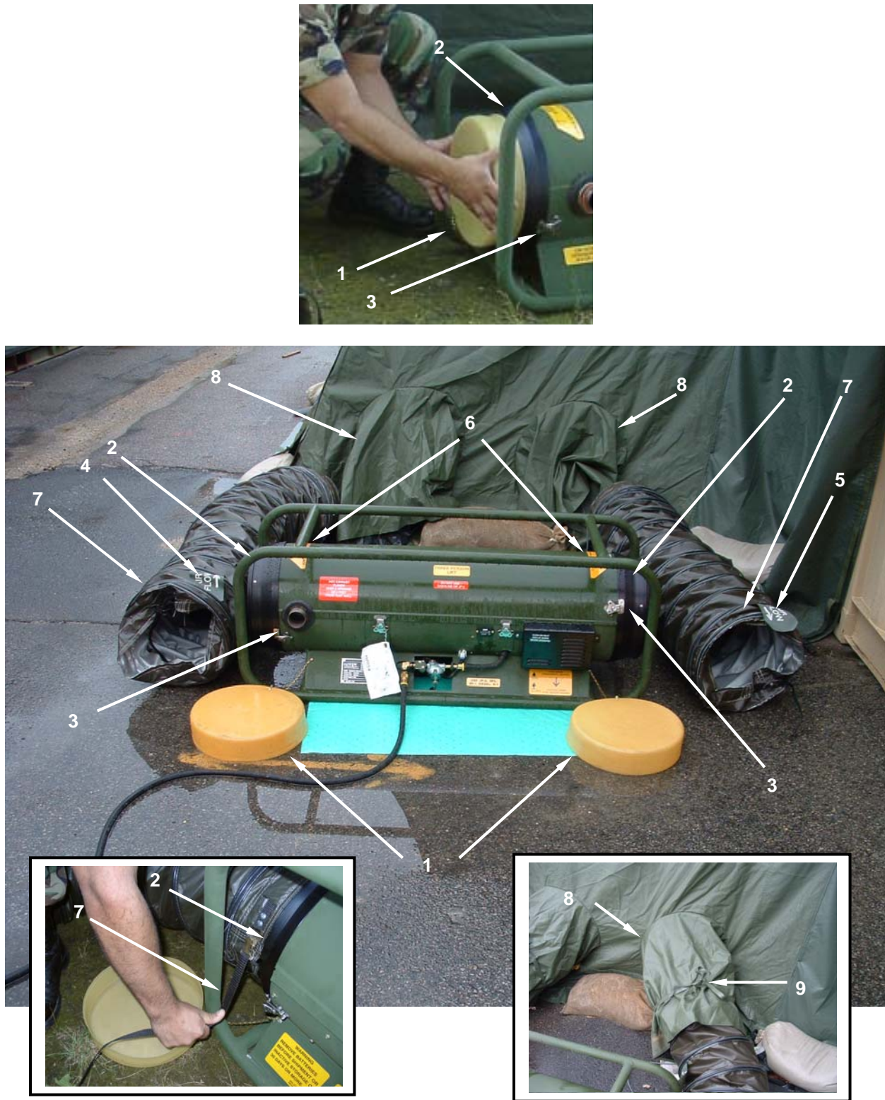
Figure 20. Installing the Air Supply and Return Ducts.
