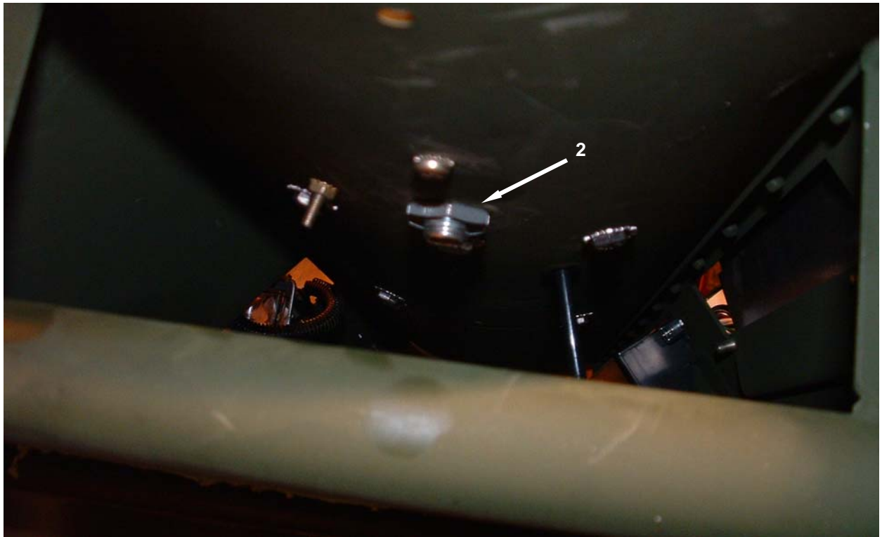
Figure 3. Replace the Float Assembly – Fuel Drain.
