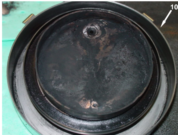
Figure 9. Replace the Burner Assembly Wick - Continued.
