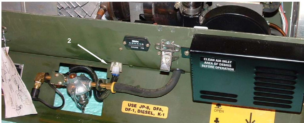
Figure 7. Replace the Electronic Box Assembly, Complete with Wire Harness – Connect Fuel Pump.
