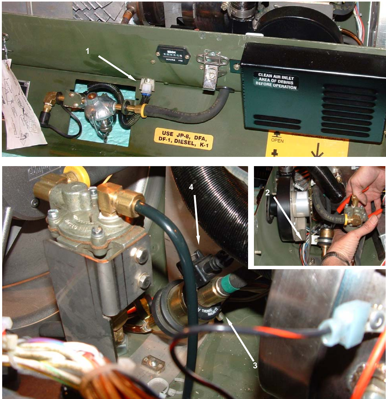
Figure 5. Replace the Electronic Box Assembly, Complete with Wire Harness – Disconnect Fuel Pump.
