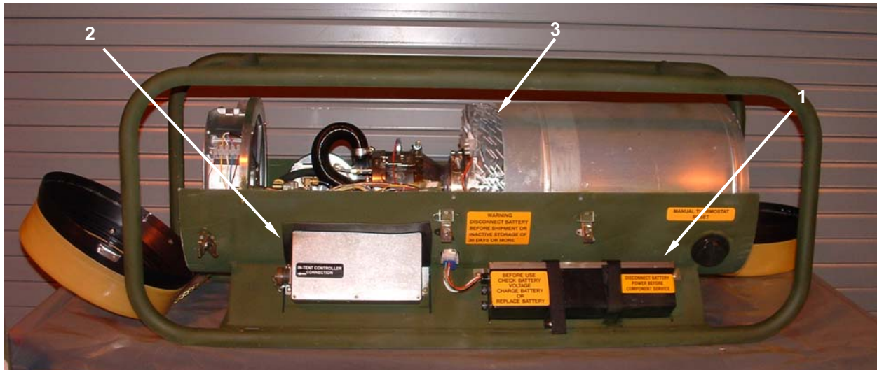
Figure 3. SHC-60K Power Control, Battery Pack and TEG.
