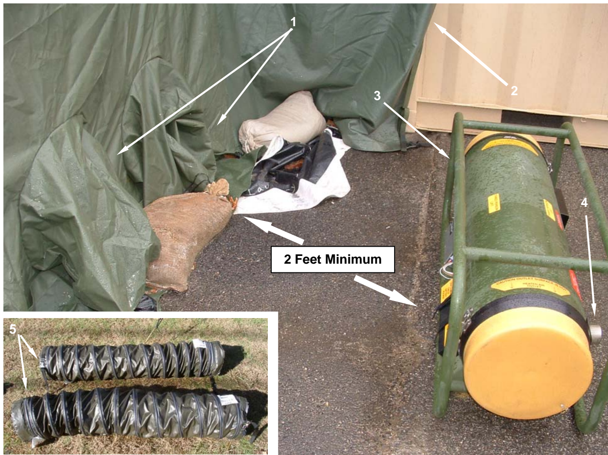
Figure 8. Positioning Heater Outside of Tent.
