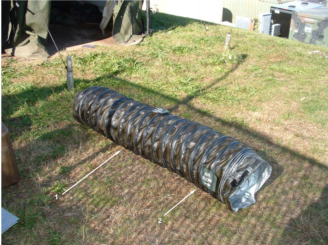
Figure 18. Air Supply and Return Ducts.
