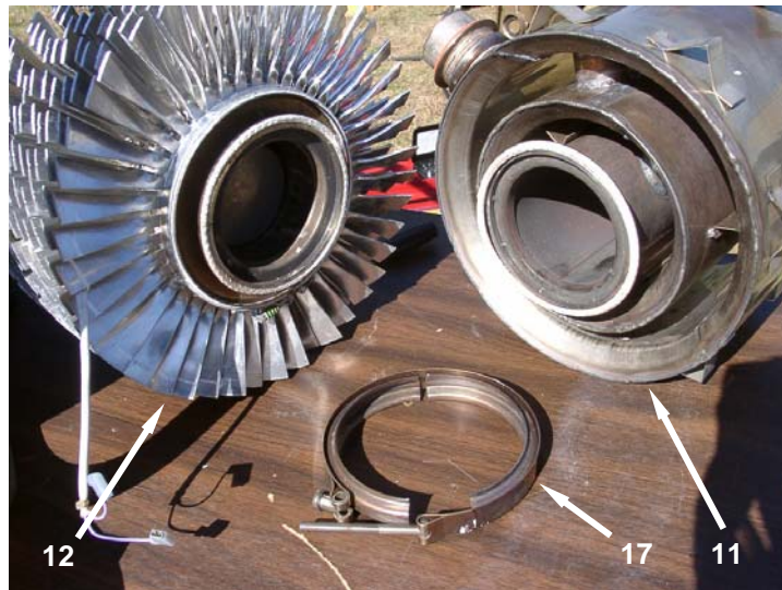
Figure 2. Remove Heat Exchanger – Continued.
