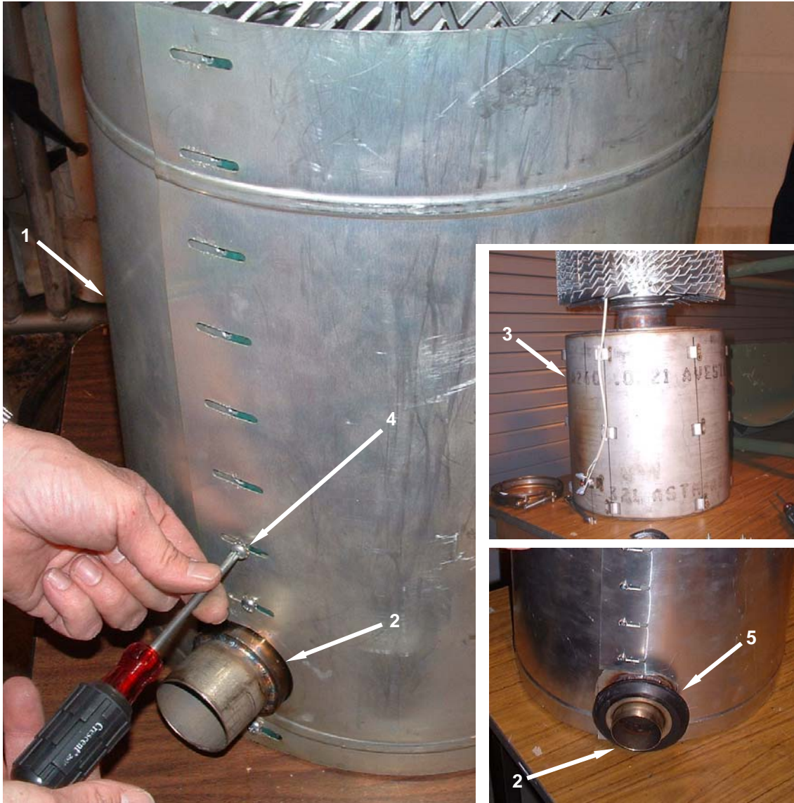
Figure 14. Install the Thermoelectric Generator – Install Wrap Cover.
