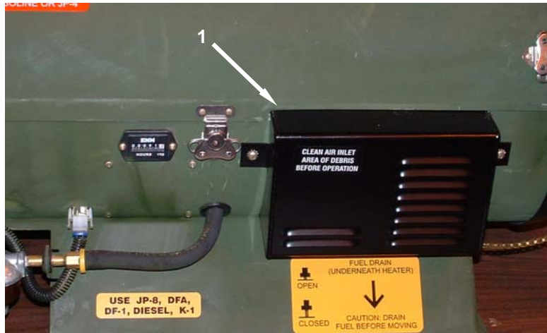
Figure 11. Replace the Electronic Box Assembly, Complete with Wire Harness – Complete Installation.
