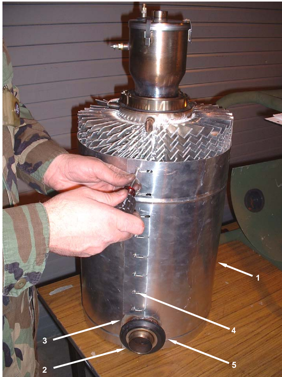
Figure 8. Replace Fin Temperature Sensor – Install Wrap Cover.
