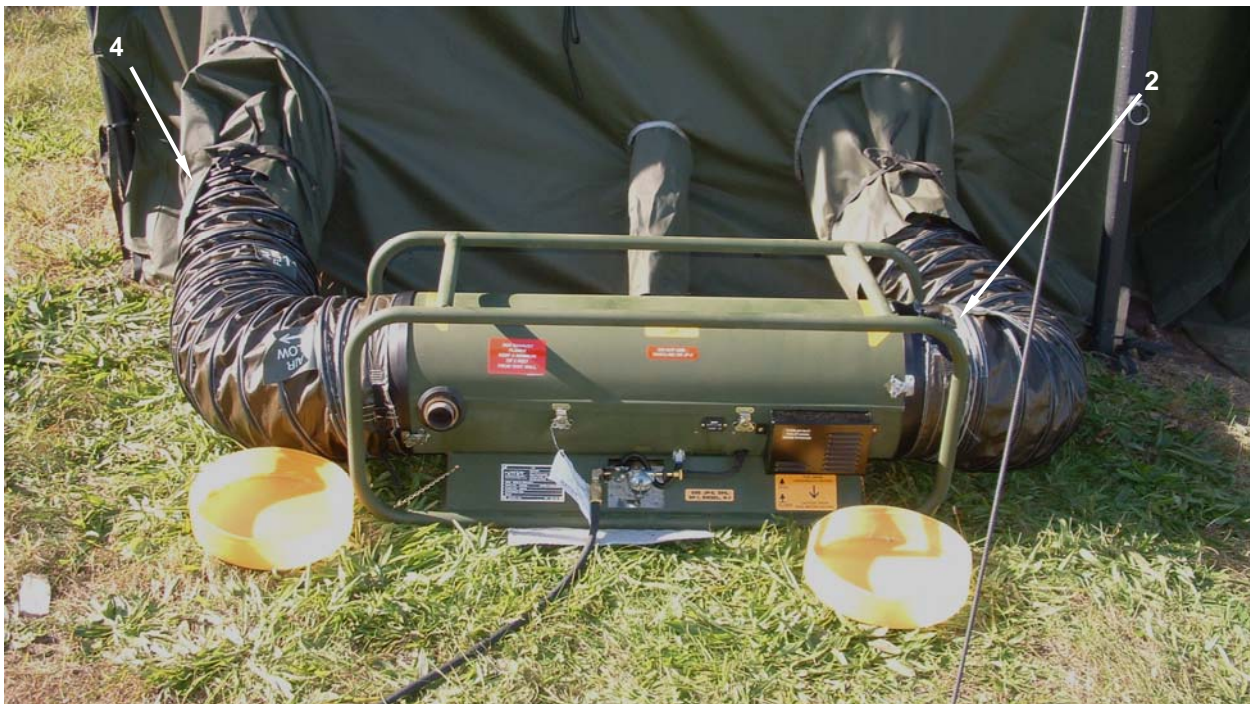
Figure 6. SHC-60K Heater Exchange Process.
