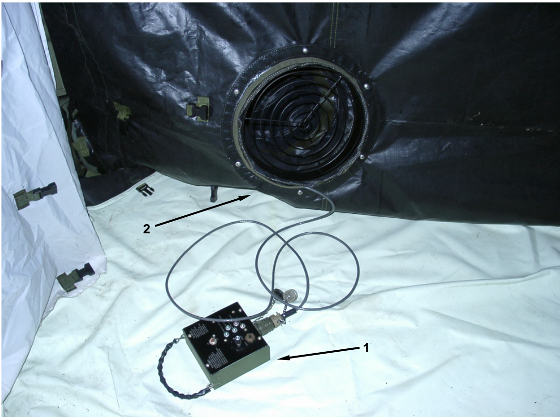
Figure 15. Route the In-tent Controller and Cable Through the Tent Duct Tunnel.
