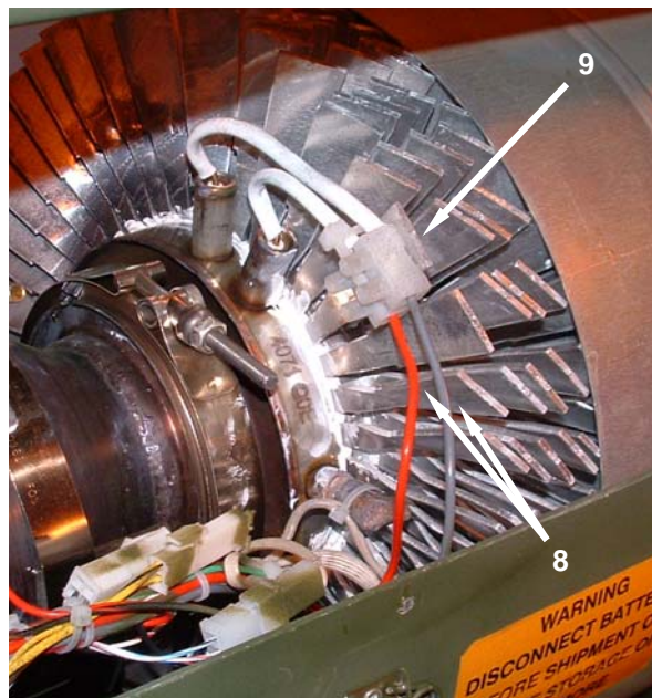
Figure 5. Replace Fin Temperature Sensor – Disassembly.
