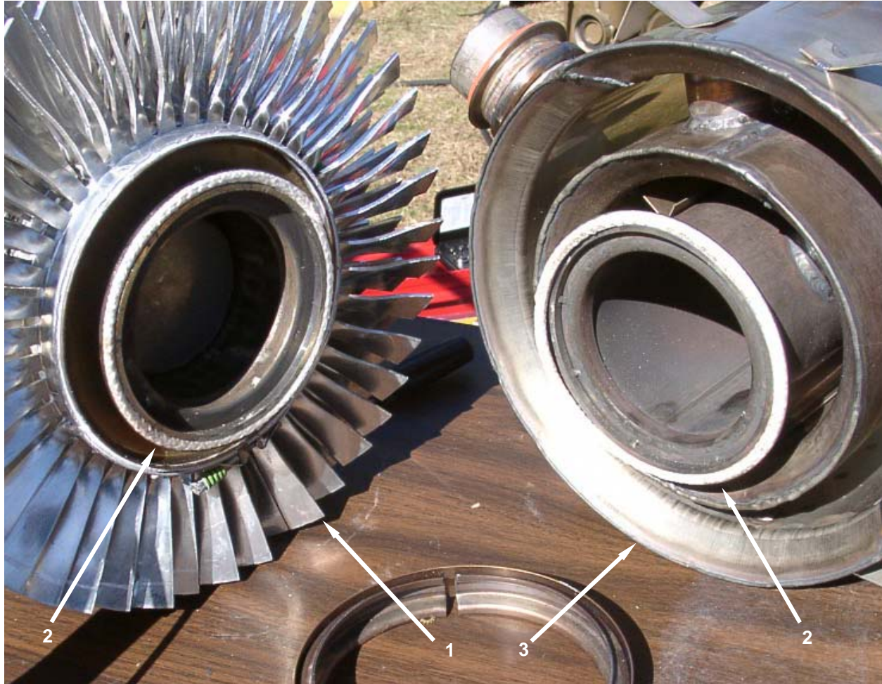
Figure 11. Install the Thermoelectric Generator – Install Fiberglass Rope.
